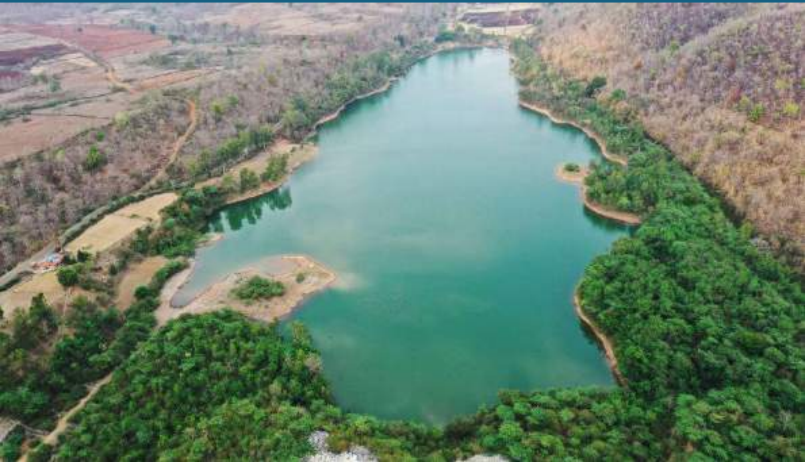
Mine Void Developed for Groundwater Recharge
